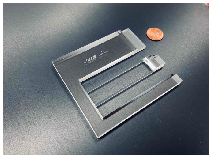
Figure 4: This photo is a resonator, another part of our sensors that move according to the vibration of the body under test.
